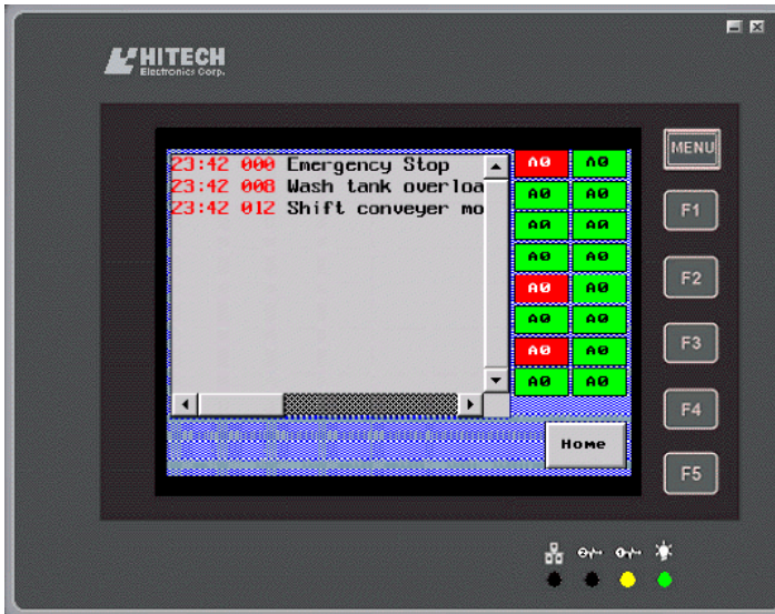
The Active Alarm List displays only the active alarms, and in numerical order.
