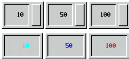
Numeric Entry buttons are used to influence Numeric Display objects.
