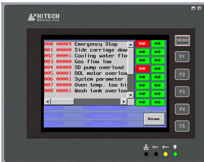
The Alarm Frequency Table displays the number of occurrences of each alarm
