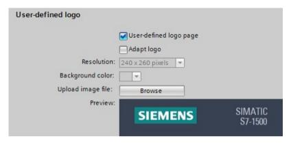
Figure 14-4 Uploading image to CPU
