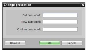
Figure 11-6 Removing know-how protection for blocks
