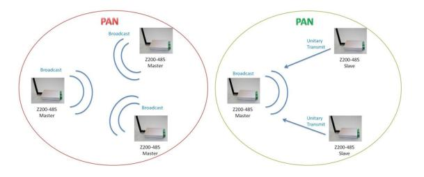
When a Master mode FBs-CMZBR sends RF packets, it broadcasts the packet to all the devices with the same PAN ID. On the other hand, when a FBs-CMZBR, as a Slave, sends data wirelessly, it only sends the data to the Master with a same PAN ID. In order for a Slave to work with a Master, user must pair each other. After successful pairing, the Slave will remember the Master' s address and will be able to send RF packet directly to the Master. d. LED display:
