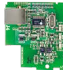
▪ CME-USB01 Second communication card (USB1.1)
