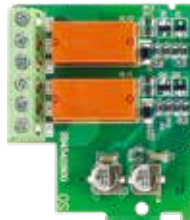
▪ EME-R2CA Relay card (2 form C/Change-over contacts)
