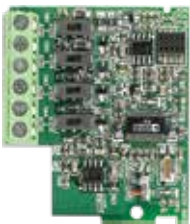
▪ EME-A22A Anglog I/O Card (12 bits)
