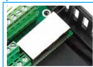
Dual RJ45 communication ports
