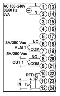
(2 sets of alarm outputs or with RS485 communication)
