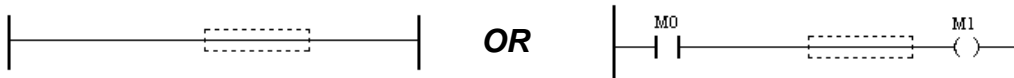
Inserting a function block into a line, or connecting a function block to a contact in series
