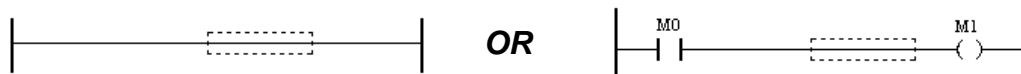
Inserting a coil into a line, or connecting a coil to a coil in parallel
