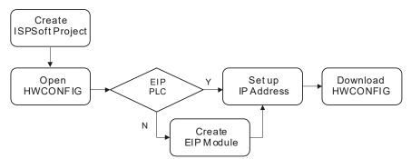
Refer to section 4.1.1 for how to set up an EIP module through the HWCONFIG in the ISPSoft.
