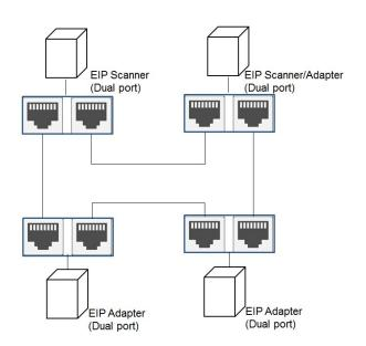
When a switch is needed for topology, the switch should support the DLR function. If not, the connection might fail.
