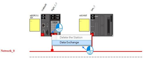
After the selection is made, the system will create a Data Mapping Tab, shown as Network\_0.
