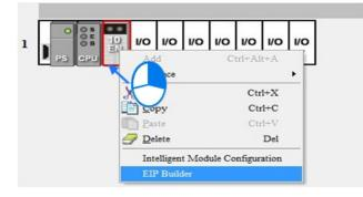
7.2 Right-click the AHCPU5x1-EN on the CPU's main backplane and you will see the EIP Builder. Double click it to open the EIP Builder.
