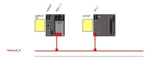
Once the connection is established, click the network line "Network\_0", you will see all the connected devices in this network.
