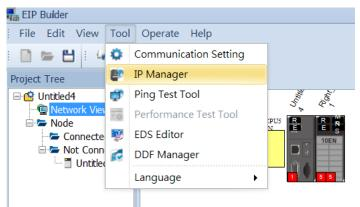
• The IP Manager can be the BOOTP/DHCP Server, receiving IP address requests from devices.
