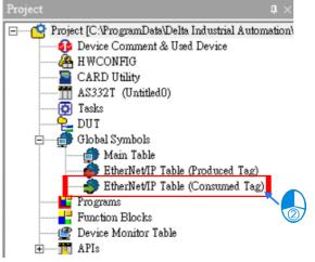
% It is only available for PLC with the EtherNet/IP TAG function. Refer to chapter 3 for EtherNet/IP specifications to learn the supported models and number of TAGs suppored.
