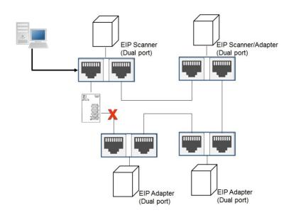
Or you can use an EIP tap to connect your PC so that the ring topology can stay intact.
