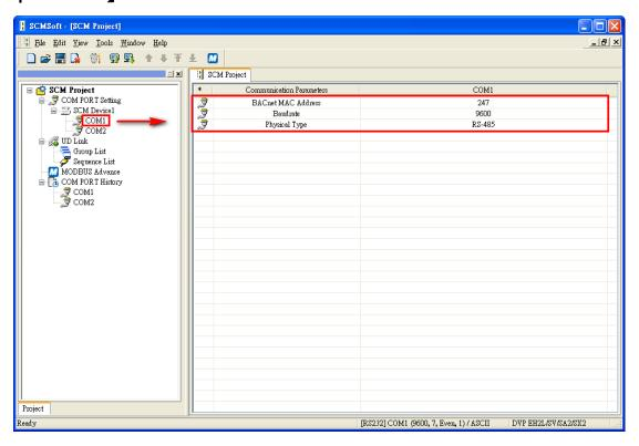
BACnet MAC address: 1 ~ 247 (Default: 247). It can not be the same as the address of other device on the BACnet network.
