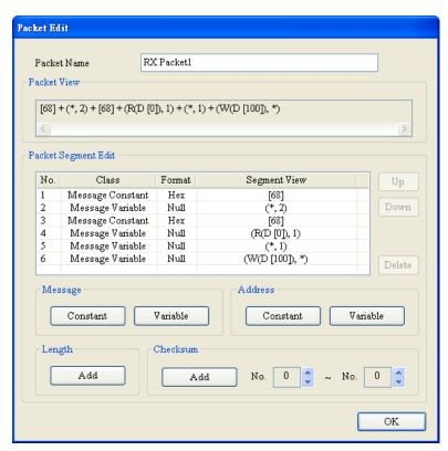
Note: Some unimportant words can be ignored. The user can just store the data which is needed in the registers (Dx), and the data whose length of the response code is unknown can be stored in the registers by means of this method.
