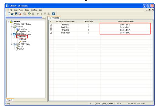
The default address is D500. The user can change the start address in MODBUS Advance.
