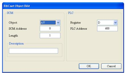
Object: The user can select "AV" or "BV". "AV" corresponds to data the registers in the PLC, and "BV" corresponds the coil in the PLC.
