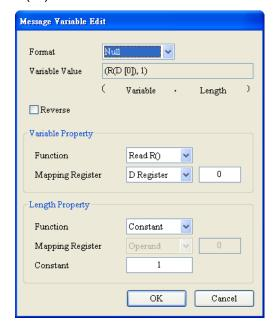
Ignore the function code (FF) of the response: (\*, 1): Ignore the word whose length is 1. If the user wants to store the function code, the user can refer to the setting of the device address (IA) to store the function code in the D register.
