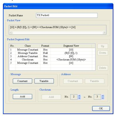
There is no response address for type 1, so the user does not need to edit the function code of the response (Rx).
