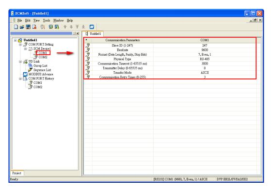
Set the communication parameters of COM1: station address 247 (default), Modbus RTU, 9600, 8, Even, 1.
