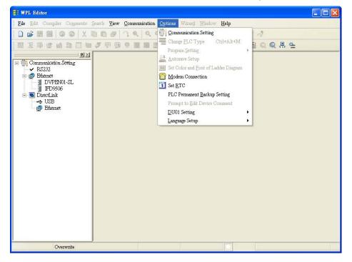
(2) Choose RS-232 in Communication Setting, designate "COMP Port", and enter the communication parameters. The communication parameters here should conform to the default setting of COM1 on the SCM module. If other communication parameters are used, they need to be modified in COM PORT Setting of the SCM module. In addition, the setting of "Station Address" should conform to COM1 on the SCM module rather than the station address of the MPU of the PLC.
