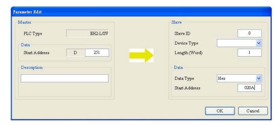
PLC (D300~D309 in the master←D100~D109 in the slave), (D350~D354 in the master→D150~D154 in the slave)
