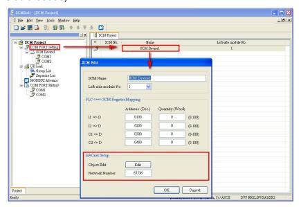
BACnet object edit: Editing the AV and BV values which correspond to the data registers and coils in the Delta PLC master connecting to the SCM module
