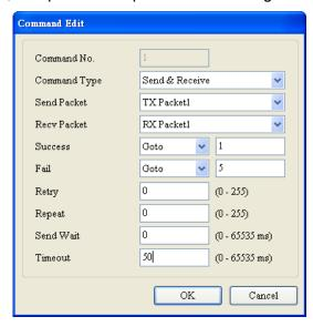
Command No.: Each command has its own number. The user can designate the sequence of executing the commands through these numbers.
