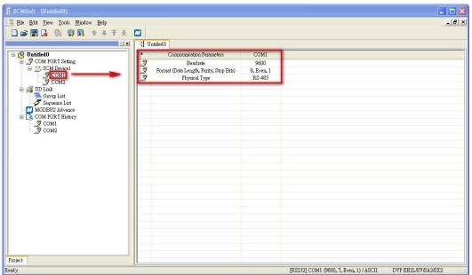
Set the communication parameters of COM1: Station address 247 (default), UD Link, 9600, 8, Even, 1.
