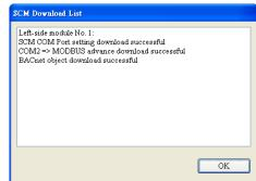
After the parameters are downloaded, the AV and BV values in the software correspond to the registers and bit in the PLC connected to the SCM module.
