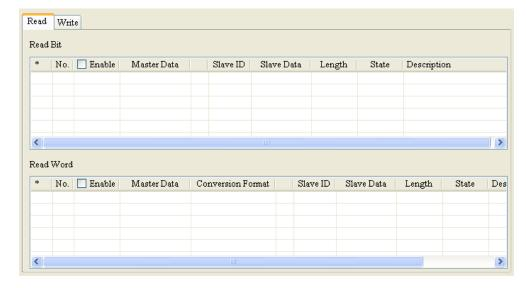
Press the right key of the mouse, and click "Add Item" to increase bits and words. The bits are listed in the upper column, and the words are listed in the lower column.
