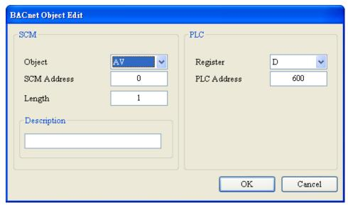
Object: The user can select "AV" or "BV". "AV" corresponds to the data registers in the PLC, and "BV" corresponds the coil in the PLC.
