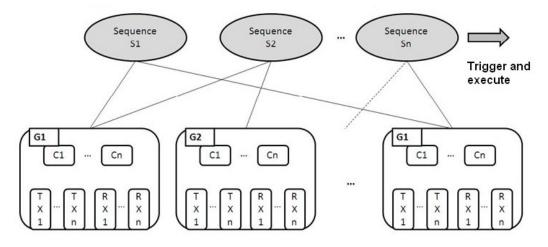
First of all, establish the transmission instructions (TXs) and the reception instructions (RXs) in the group. Then, set the execution sequence and the number of times for TXs and RXs through the commands. Finally, trigger and execute the instructions as a group. In addition, if various groups of group packets are required in a large system, the user can create the groups in the sequences, and set the execution sequence.
