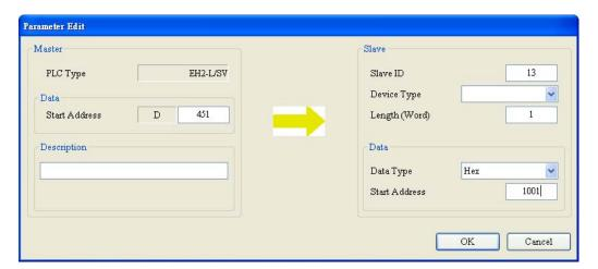
After the setting is complete, the user can designate the communication port using MODBUS Advance — COM port 2 on the first left-side module.
