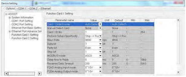
(a) When the function card is an AS-F232, AS-F422, or AS-F485, configure the communication settings in the red box.
