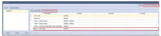
The mapped register for **Port 1- 4 Pin2 value** of **Normal Exchange Area** is D29029. For the pin2 input value, the addresses D29029.0~ D29029.3 correspond to port 1~ port 4 respectively.
