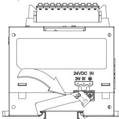
■ Use screws to secure the baffle.
