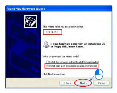
The path C:\Program Files\Delta Industrial Automation\ISPSoftx.xx\drivers\Delta\_PLC\_USB\_Driver shown in the picture below is the folder where the software is installed. If the path is modified, please select the folder where the software will be installed.
