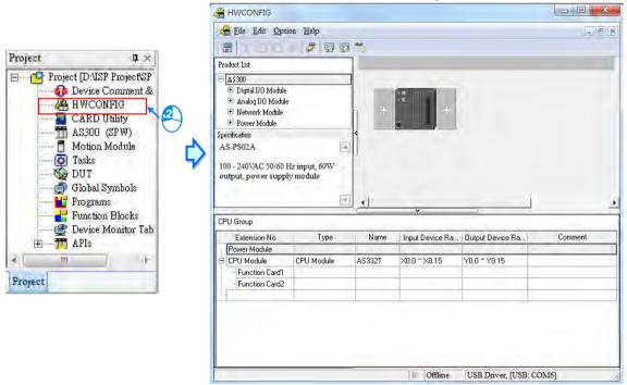
Users can configure the hardware according to the information above. After users type "SPW PLC Control Station", the project can be shared.
