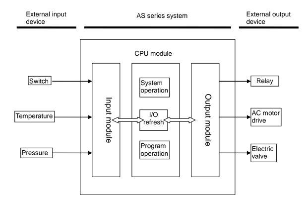
The operation of the CPU module is illustrated above. The system procedures related to the initialization, the diagnosis, and the communication, and the program procedures related to the external interrupts and timed interrupts are simplified. Users can refer to other manuals for more information. The operation of the CPU module is described below.
