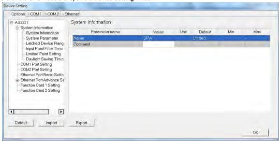
Type "SPW PLC" in the **Name** box, and then type "The example in AS300 Quick Start" in the **Comment** box. Finally, click **OK**, and close the window.
