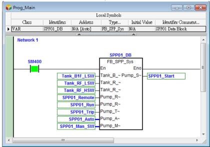
If users want to alter the value in the device, they can click the right mouse button. Tank\_B1F\_LSW is the device which is modified here. Please notice that the device corresponds to an actual I/O device. Setting the device to ON or OFF is meaningless because the actual I/O value covers the setting value immediately. To alter the value in the device, users need to force the device ON or OFF.
