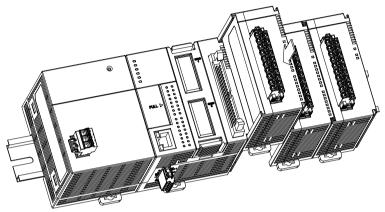
If there is a vibration source in the installation site, it is suggested to installed anti-vibration baffles on the sides of the AS series for better stabilization as the gray baffles illustrated below.
