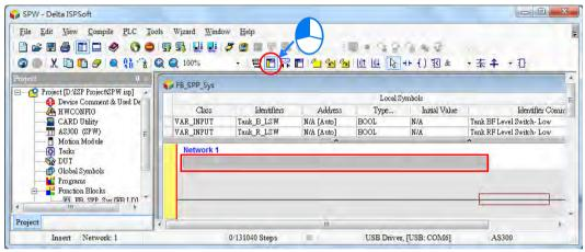
Type the following description as the comment on network 1. If users want to start a new line of text at a specific point, they can press Alt+Enter on the keyboard.
