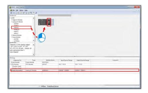
In order to complete the basic setting, users need to set the relation between the signals and the conversion values for the analog module. Double-click the module to open the **Device Setting** window.
