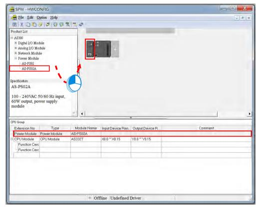
After the module is placed in the appropriate position, the system automatically distributes the addresses to the module. The default addresses are IN: D28000~D28009 / OUT: D28010~D28019. (IN: D28000 is the module state; D28002~D28003 is the device range for channel 1AD, D28004~D28005 for channel 2AD; D28006~D28007 for channel 3AD; D28008 ~ D28009 for channel 4AD.) (OUT: D28010~D28011 is the device range for channel 1DA; D28012~D28013 for channel 2DA)
