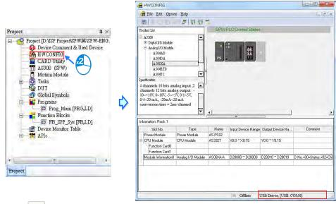
After users click , the **Transfer Items** window will appear. After the users click **OK**, the hardware configuration and the CPU parameters will be downloaded to the CPU module.
