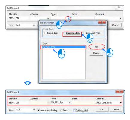
After the local symbol is created, the identifier can be given to the function block. (The data type should be the same with the name of the function block.)
