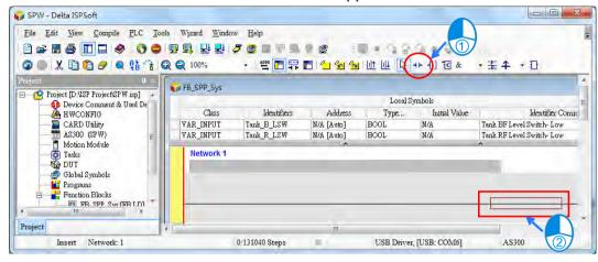
Click ???, and type "Pump\_Remote". When "Pump\_Remote" is typed, the drop-down list appears. Users can select the item directly, or type the words by themselves. After "Pump\_Remote" is typed, press the enter key. (If the address appears, users can click to switch the mode. In either mode, users can use the words or the addresses when they write the program.)
