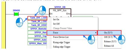
The value in the device is altered, and a lock symbol indicating that the device is forced ON appears.
