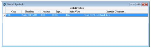
Users can create the global symbols for the data in the table above in the same way. (For the analog module, the data type is a real floating-point number. Therefore, the symbol occupies two data registers, and the address in the **Address** box is the initial address.)
