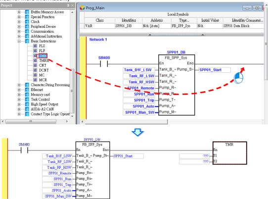
If users need to create the second system, they only need to call "FB\_SPP\_Sys" again, and type the identifier. Please notice that the same data block can not be used in the two systems unless user consider that the value of VAR\_OUTPUT and that of VAR of in the first system does not affect those in the second system. Otherwise, please create a new identifier for the second system, as shown below.
