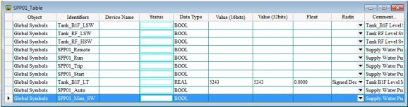
If users want to alter the value in the device, they can click the right mouse button. The state of SPP01\_Man\_SW is altered here. Owing to the fact that the device does not correspond to an actual I/O device, users can set the device to ON or OFF.
