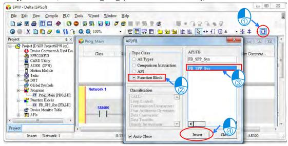
After the function block interface appears, type the identifiers as shown below.
