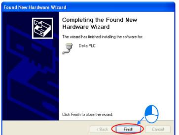
After the software is installed, users can see the USB driver in the **Device Manager** window. (The COM number of the USB may vary from computer to computer.)
