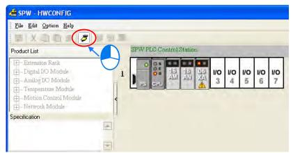
Generally speaking, a hardware configuration error occurs if the BUS FAULT LED indicator on the CPU module is ON. Users can select AH06XA-5A, click the right mouse button, and select **Diagnosis**.
