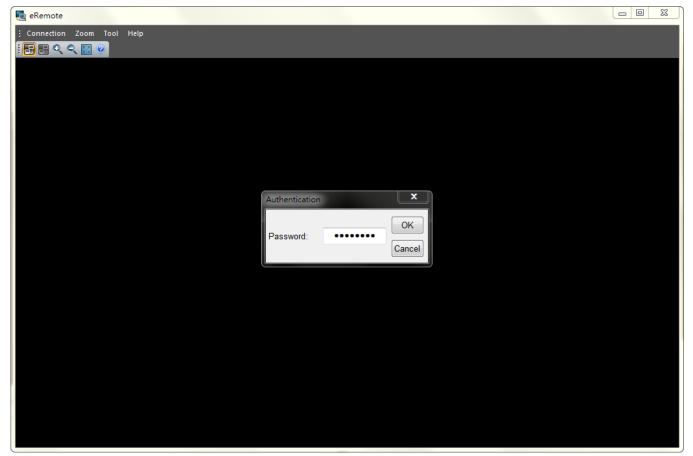
After entering the correct password, the system will start the connection automatically. After the connection is successfully established, the users can monitor and control HMI screens on the computer screen.
