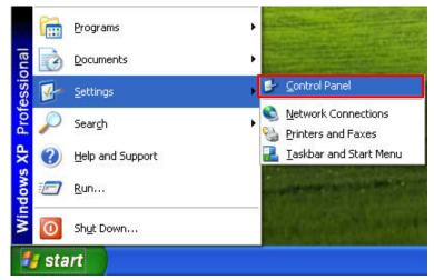
Power on PC and start Windows. Click **Start > Programs**, point to **Control Panel**, and then select **Network Connections**.
