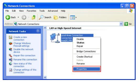
The Local Area Connection Properties dialog box will open. Use General tab to select Internet Protocol (TCP/IP). Then, press Properties button.
